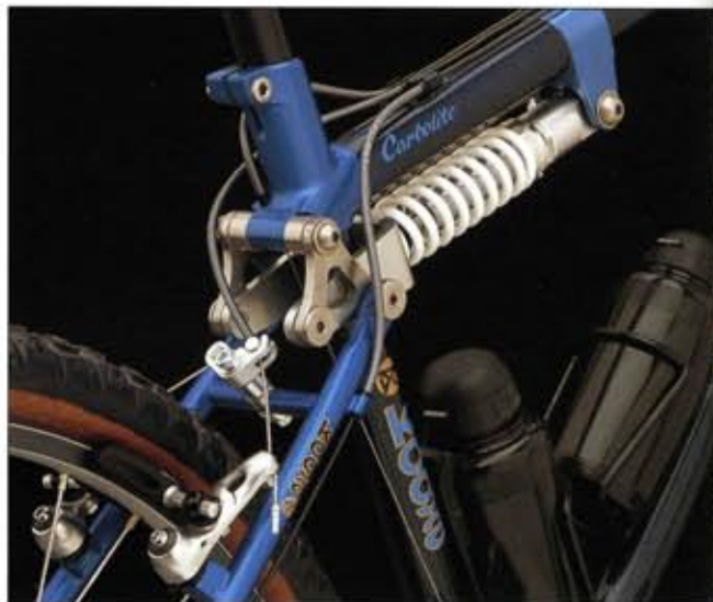
Koga-Miyata's instelbare suspensie systeem (RDG-S).
